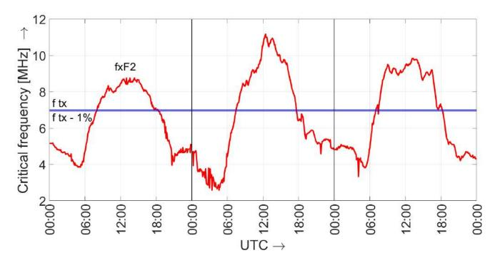
The transmit frequency  $f_{tx}$  is fixed, and fxF2 is variable.
