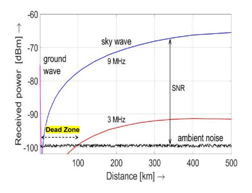
Simulated signal strength using <u>real</u> antennas
