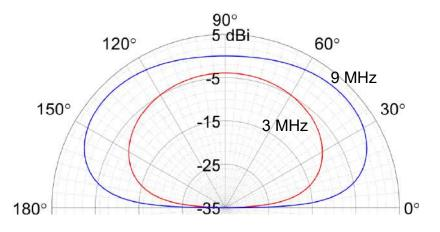
Antenna gain versus elevation angle
